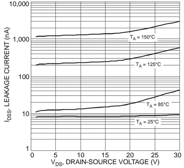
Fig. 10 Typical Leakage Current vs. Drain-Source Voltage
