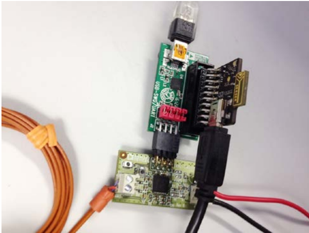
Figure 3. EVAL-CN0300-EB1Z Board Connected to the USB-SWD/UART Board and SEGGER J-Link-Lite Board
