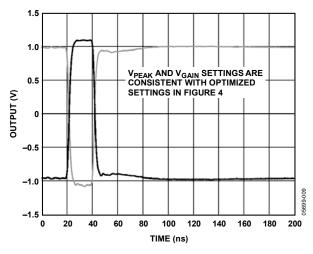
Figure 10. Equalized Pulse Response for 100 M of Cable
