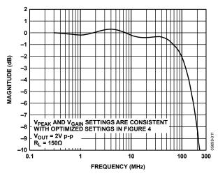
Figure 8. Equalized Frequency Response for 100 M Cable
