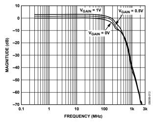
Figure 6. Frequency Response for Various V<sub>GAIN</sub> Settings Without Cable
