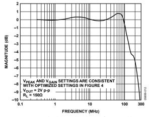
Figure 7. Equalized Frequency Response for 50 M Cable
