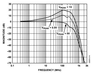
Figure 5. Frequency Response for Various VPEAK Settings Without Cable
