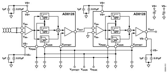
Figure 21. Cascaded AD8128 Configuration
