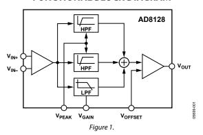
Low integrated output noise and offset voltage adjust make the AD8128 an excellent choice for dc-coupled wideband RGB-over-CAT-5 applications. For systems where the UTP cable is longer than 100 meters, two AD8128s can be cascaded to compensate for up to 200 meters of CAT-5/CAT-5e.
