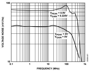
Figure 12. Voltage Noise vs. Frequency
