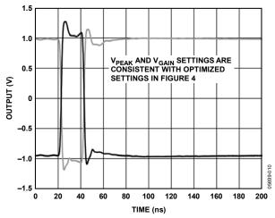
Figure 9. Equalized Pulse Response for 50 M of Cable
