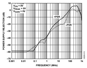
Figure 16. Power Supply Rejection vs. Frequency
