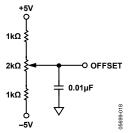
Figure 20. Circuit to Control V<sub>OFFSET</sub> (±2.5 V)
