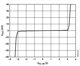
Figure 11. Output Voltage vs. Common-Mode Input Voltage
