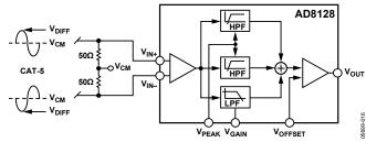
Figure 18. Single Receiver Configuration for CAT-5 Equalizer
