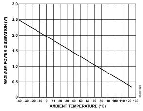
Figure 2. Maximum Power Dissipation vs. Temperature
