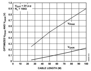
Figure 4. V<sub>PEAK</sub> and V<sub>GAIN</sub> Settings vs. Cable Length
