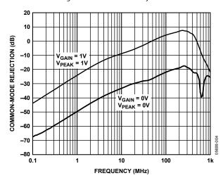
Figure 15. Common-Mode Rejection vs. Frequency
