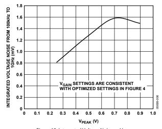
Figure 13. Integrated Voltage Noise vs. VPEAK
