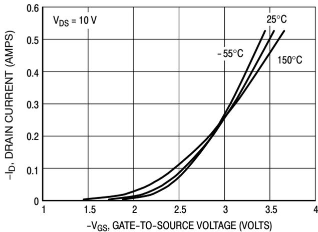
Figure 1. Transfer Characteristics
