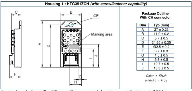
Housing 1 can be fixed with a M2 screw. The recommended maximum mounting torque is 0.22 Nm.
