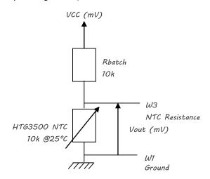
$$V_{OUT}(mV) = \frac{Vcc(mV) * NTC_{HTG3500}(\Omega)}{R_{batch}(\Omega) + NTC_{HTG3500}(\Omega)}$$
