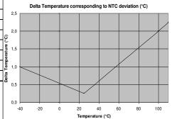
0.1°C tolerance on Resistance Measurement
