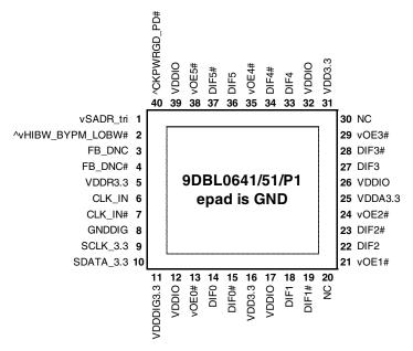
40-VFQFPN, 5mm x 5mm 0.4mm pin pitch ^ prefix indicates internal 120KOhm pull up resistor ^v prefix indicates internal 120KOhm pull up AND pull down resistor (biased to VDD/2) v prefix indicates internal 120KOhm pull down resistor
