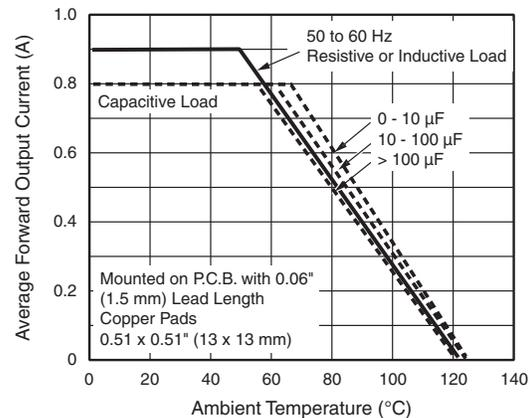
Fig. 2 - Derating Curves Output Rectified Current for B250C800D...B360C800DM
