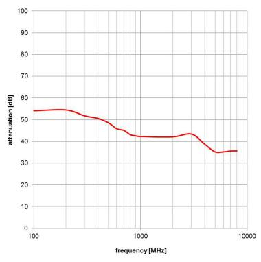
measurement based on assembeled top cover with SMD frame according to IEEE STD 299
