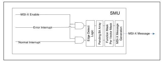
To signal an Interrupt with MSI-X enabled, a memory write transaction will be created using the Message Address and the Message Data of the associated entry.
