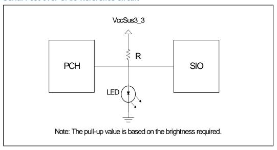
The anticipated usage model is that either the PCH or the SIO can drive a pin low to turn off an LED. In the case of the power LED, the SIO would normally leave its corresponding pin in a high-Z state to allow the LED to turn on. In this state, the PCH can blink the LED by driving its corresponding pin low and subsequently tri-stating the buffer. The I/O buffer should not drive a '1' when configured for this functionality and should be capable of sinking 24 mA of current.
