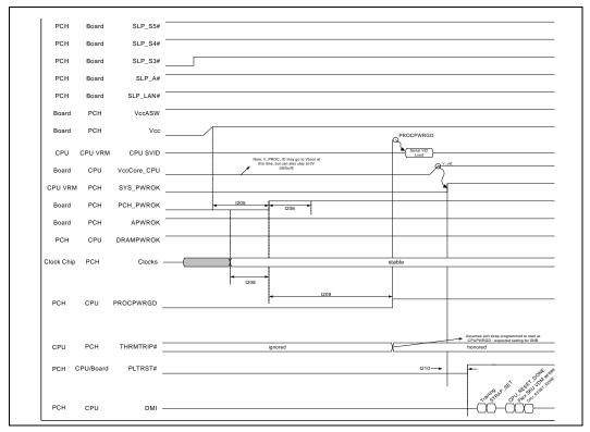
Figure 8-5. S5/Moff - S5/M3 Timing Diagram
