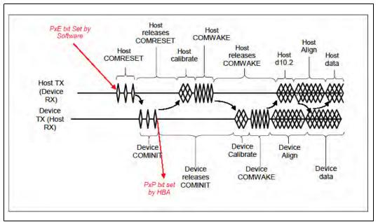
Figure 5-10. Flow for Port Enable / Device Present Bits
