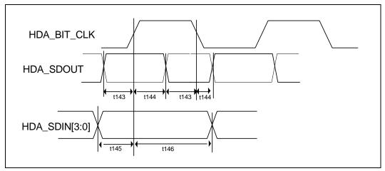
Figure 8-24. Transmitting Position (Data to Strobe)
