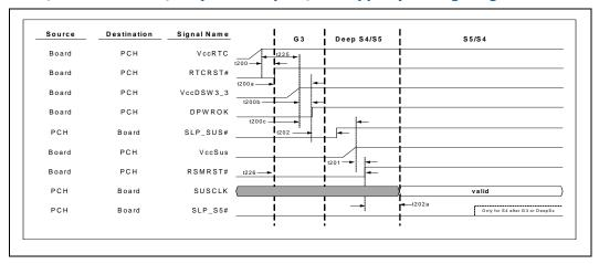
Figure 8-2. G3 w/RTC Loss to S4/S5 (Without Deep S4/S5 Support) Timing Diagram
