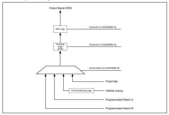
Figure 5-25. SGPIO Output OD1 Signal
