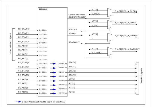
Figure 5-28. SCU SGPIO Unit Pin Mapping
