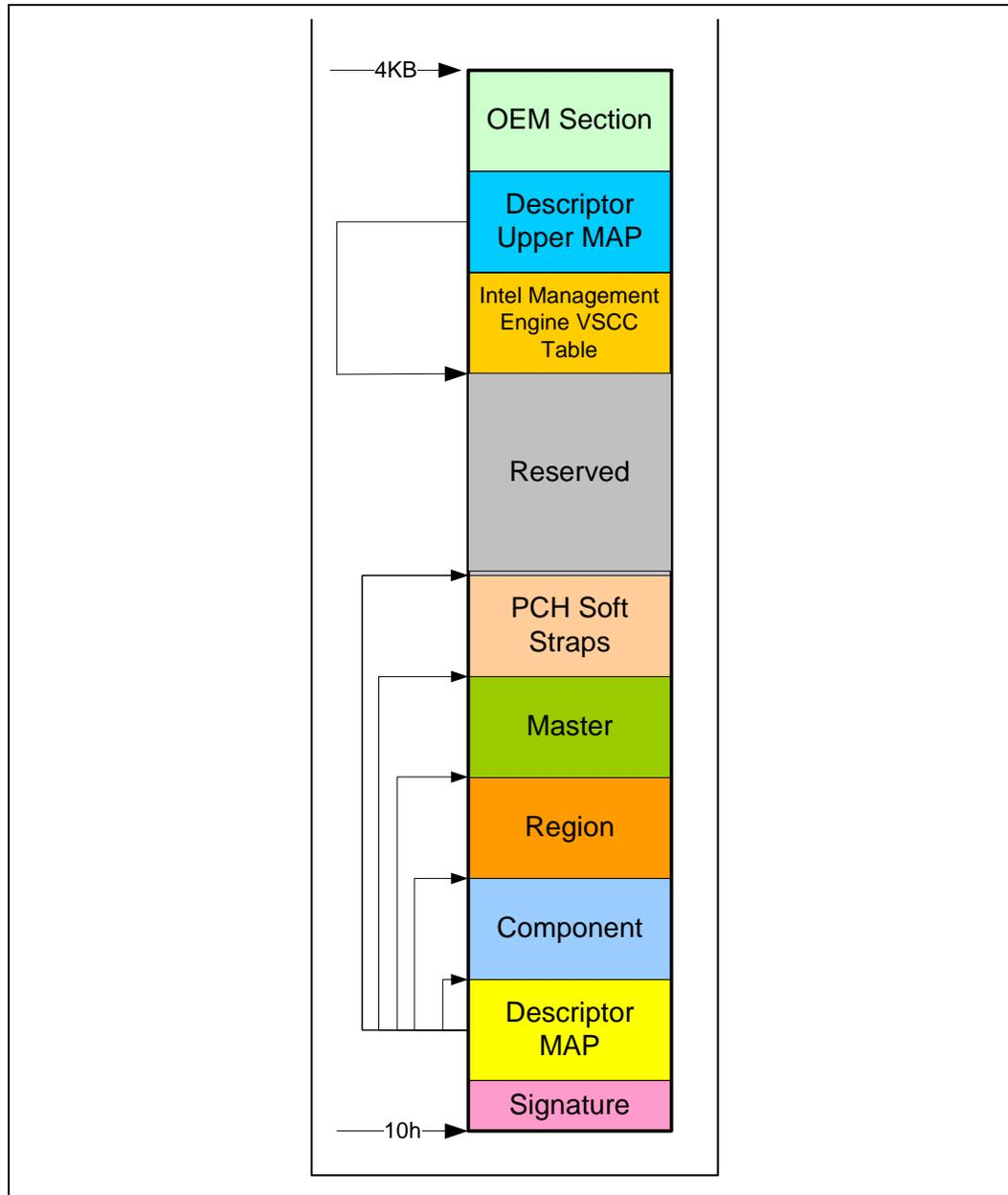
1. The Flash signature selects Descriptor Mode as well as verifies if the flash is programmed and functioning. The data at the bottom of the flash (offset 10h) must be 0FF0A55Ah in order to be in Descriptor mode.
