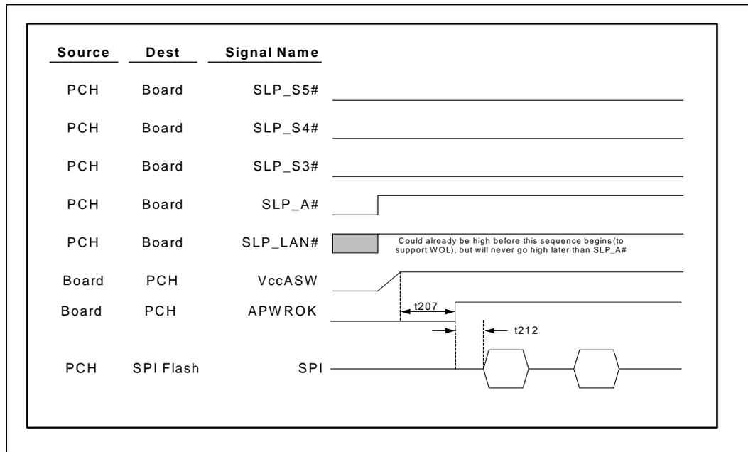
Figure 8-6. S0 to S5 Timing Diagram
