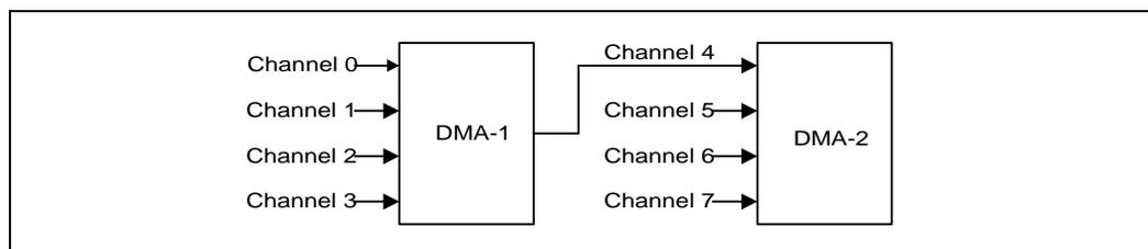
Each DMA channel is hardwired to the compatible settings for DMA device size: Channels [3:0] are hardwired to 8-bit, count-by-bytes transfers, and Channels [7:5] are hardwired to 16-bit, count-by-words (address shifted) transfers.
