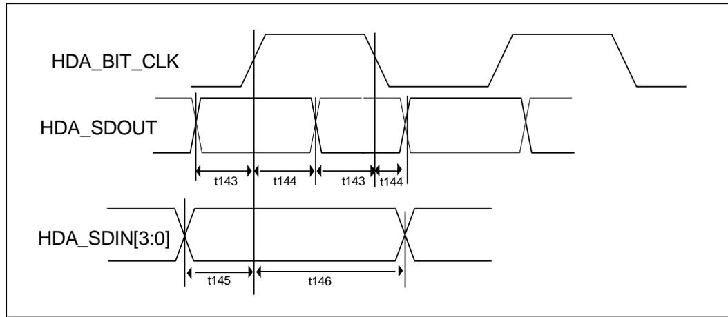
**Figure 8-24. Transmitting Position (Data to Strobe)**
