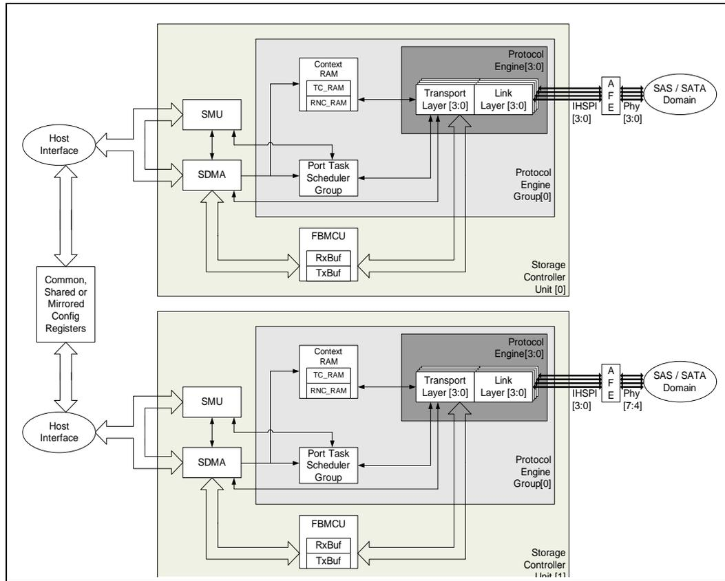
The Dual SCU-4 appears to the Driver as SCU[0] + SCU[1] behind a common PCIe function. Both SCUs are mapped behind a common set of PCIe BARs. Each SCU contains a single PEG. Note that on SCU[1] the Phys are numbered 4 thru 7 and the PEG is numbered as PEG[0].
