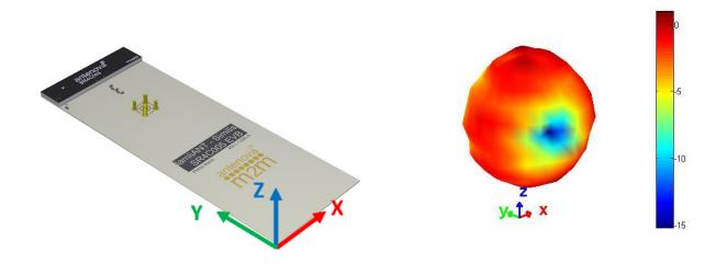
**3D pattern at 880 MHz**Drag to rotate pattern and PCB by using Adobe Reader
