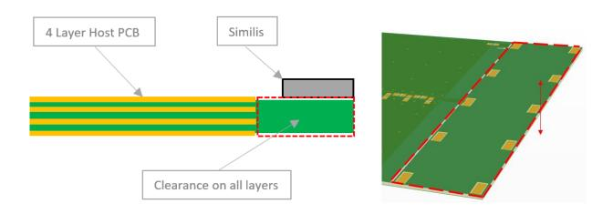
Placement of components and GND with traces adjacent to the antenna should maintain a minimum clearance of 15mm from either side. The antenna should be therefore placed in the corner to only have one side effected.
