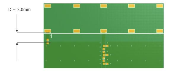
The distance D is the gap required from the antenna SMD pad edge to the ground plane. This should be maintained along the edge the antenna is placed.
