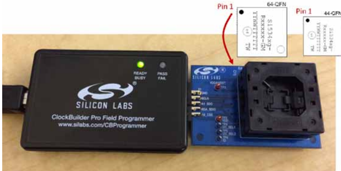
Figure 30. Correct Orientation of Device in Socket
