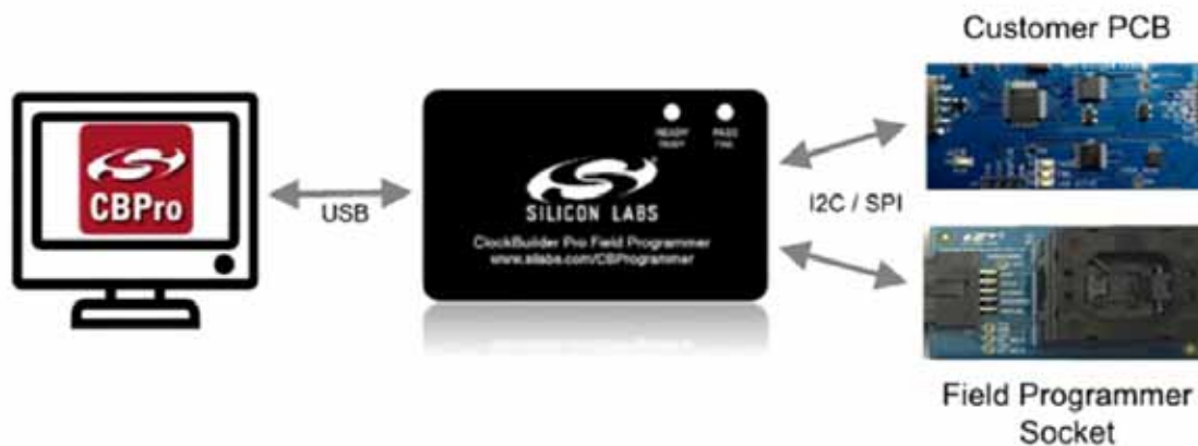
Figure 5. PC to CBPROG-DONGLE Connection
