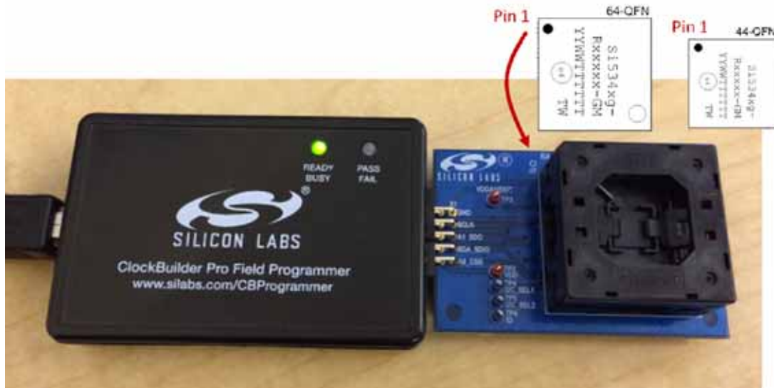
Figure 30. Correct Orientation of Device in Socket
