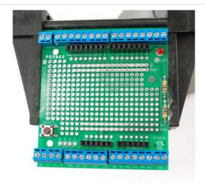
Last we will place the reset switch. This switch will let you easily reset the Arduino.
