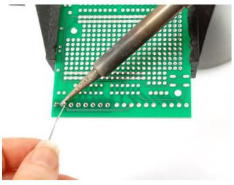
And solder the pins to the pads. Use plenty of solder so that you get the pads completely filled.
