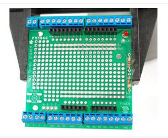
Next we will place the two 1.0Kohm resistors. These resistors are used to set the brightness of the LEDs. If you want brighter LEDs you can substitute 220 ohm resistors. If you want dimmer LEDs, you can use 4.7Kohm.
