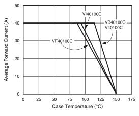
Fig. 1 - Forward Current Derating Curve
