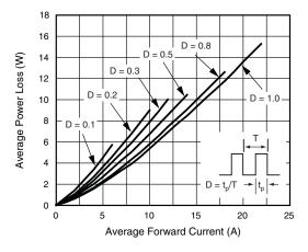
Fig. 2 - Forward Power Loss Characteristics Per Diode
