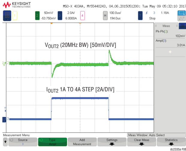
Figure 8. V_{OUT2} Transient Response at V_{IN2} = 12V , V_{OUT2} = 3.3V
