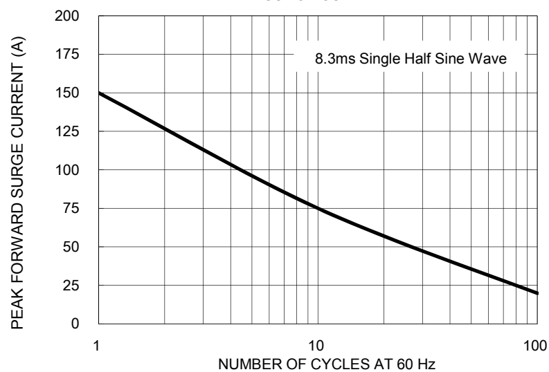
FIG. 3 MAXIMUM NON-REPETITIVE FORWARD PEAK SURGE CURRENT
