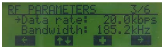
Figure 9. Menu Page: RF Parameters 3/6 (Modulation is OOK)
