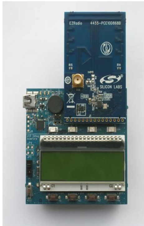
Figure 3. LCD Baseboard with Connected RF Pico Board
