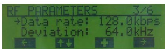
Figure 8. Menu Page: RF Parameters 3/6 (Modulation is 2GFSK)
