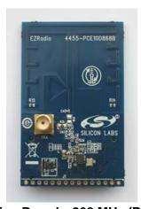
Figure 2. Si4455 RF Pico Board—868 MHz (P/N 4455-PCE10D868B)
