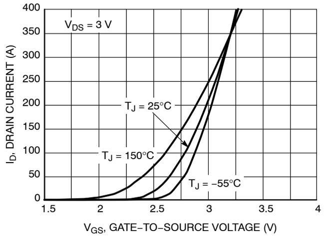
Figure 2. Transfer Characteristics
