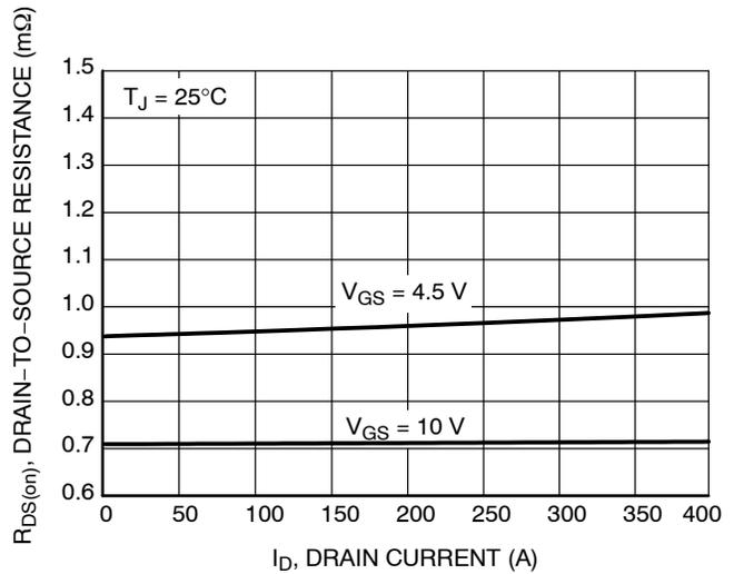
Figure 4. On-Resistance vs. Drain Current and Gate Voltage
