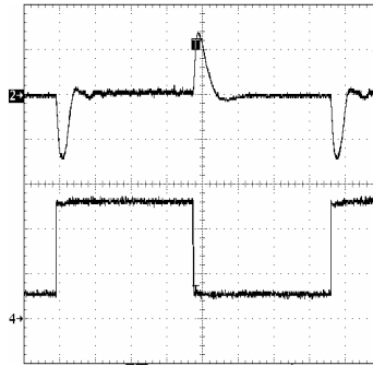
Figure 22. Optimum, R_C Is Ideal
