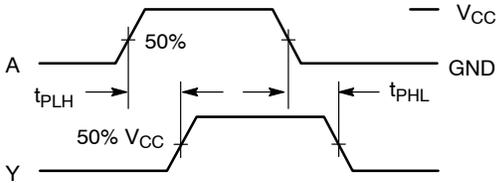
**Figure 4. Switching Waveform**
