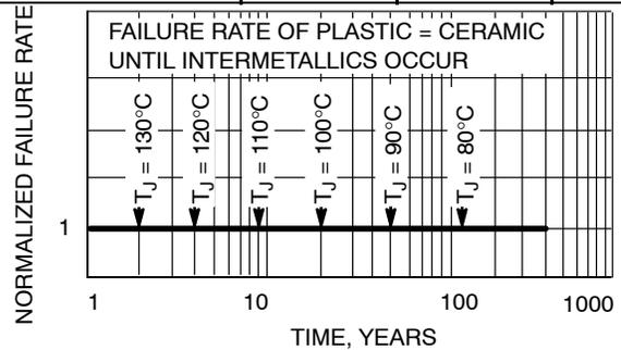
**Figure 3. Failure Rate versus Time Junction Temperature**
