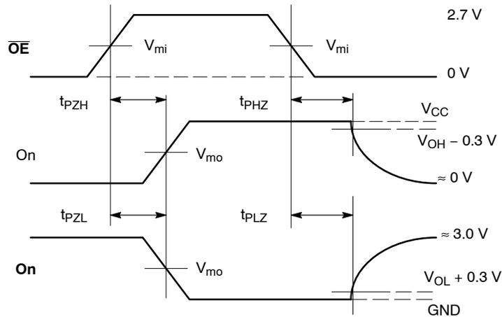
**Figure 8. AC Output Enable and Disable Waveform**
