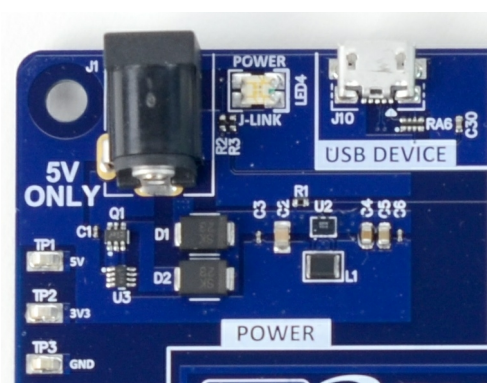
Figure 4: Power Section of Main Board
