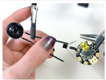
Set up the speaker in your helping hand tool and position one of its wire leads next to the transistor lead on the right.
