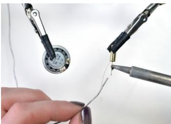
Place the small speaker and tilt ball switch in the jaws of a helping hand tool.
