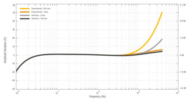
This data was generated with an aluminum unit (gray) bolted with 100 in-oz torque, and a polycarbonate unit (orange) mounted with double sided tape.
