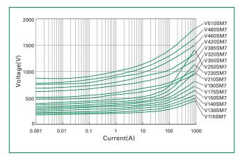
NOTE: If pulse ratings are exceeded, a shift of  $V_{N(DC)}$  (at specified current) of more than  $\pm 10\%$  could result. This type of shift, which normally results in a decrease of  $V_{N(DC)}$ , may result in the device not meeting the original published specifications, but it does not prevent the device from continuing to function, and to provide ample protection.
