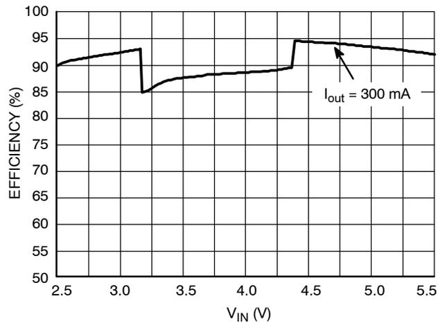
Figure 2. Efficiency vs. V<sub>in</sub> Voltage
