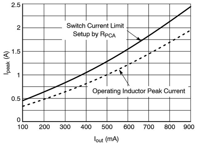
**Figure 23. Inductor Peak Currents Vs.  $I_{OUT}$  (mA)**
