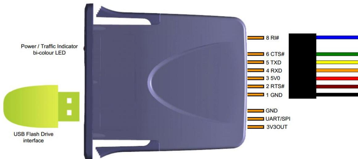
**Figure 3.1 – VDrive3 Pin Out (in UART mode)**
