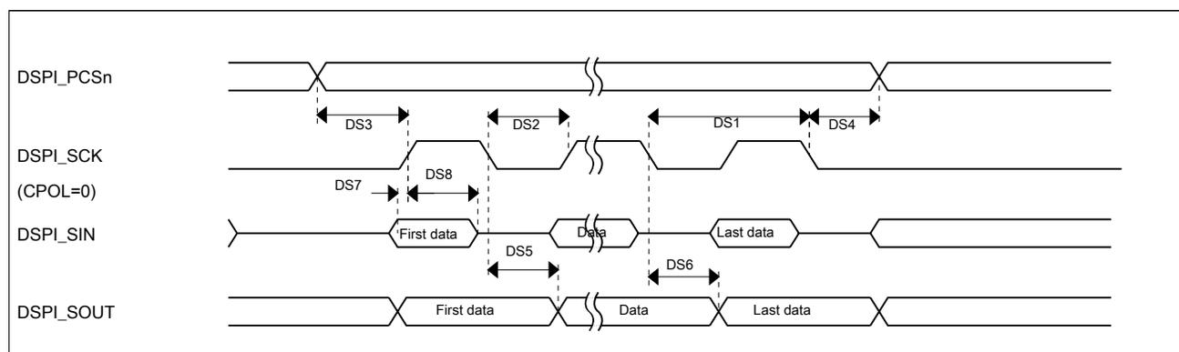
**Figure 26. DSPI classic SPI timing — master mode**
