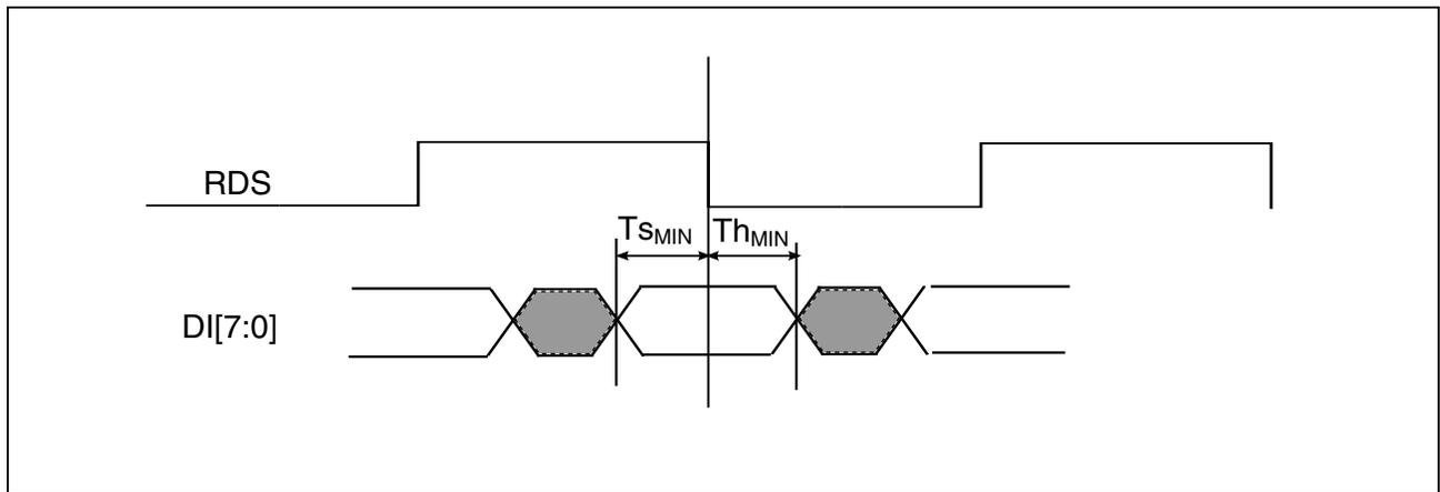
**Figure 14. QuadSPI input timing (Hyperflash mode) diagram****Table 28. QuadSPI input timing (Hyperflash mode) specifications**
