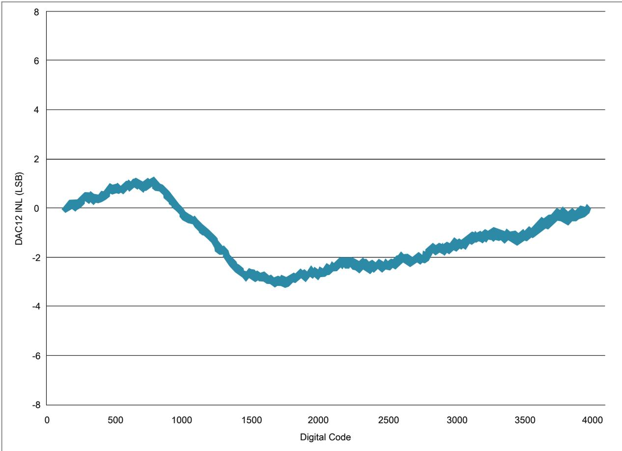
**Figure 24. Typical INL error vs. digital code**
