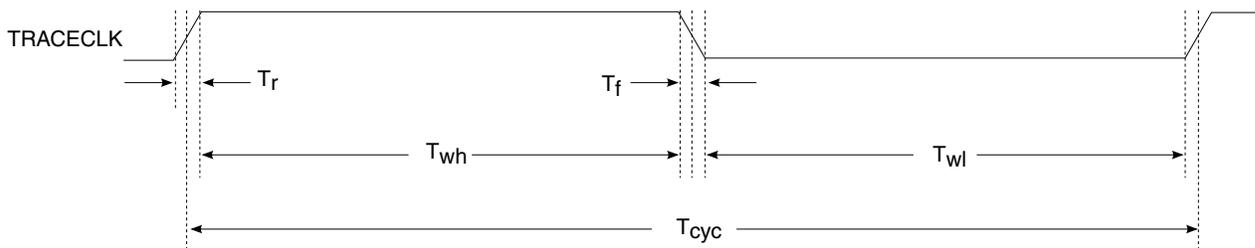
Figure 4. TRACE\_CLKOUT specifications
