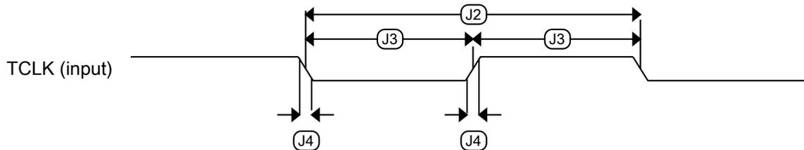
**Figure 6. Test clock input timing**
