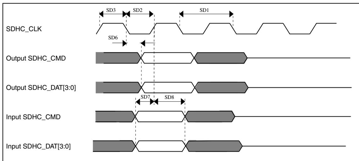
Figure 31. SDHC timing
