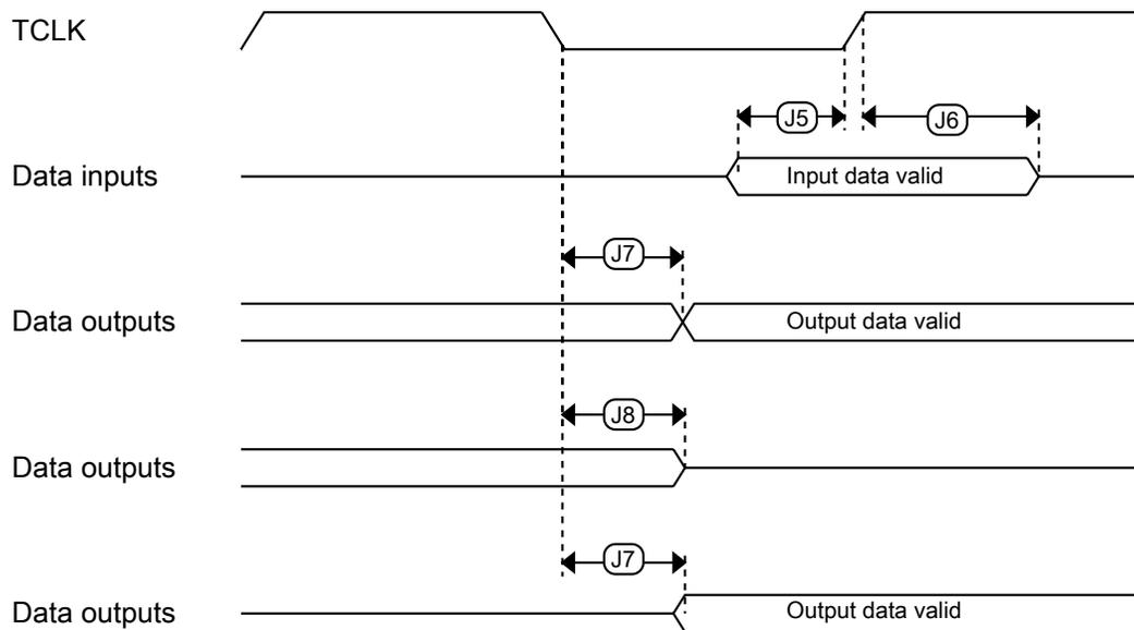
**Figure 7. Boundary scan (JTAG) timing**
