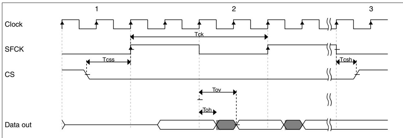
Figure 13. QuadSPI output timing (DDR mode) diagram
