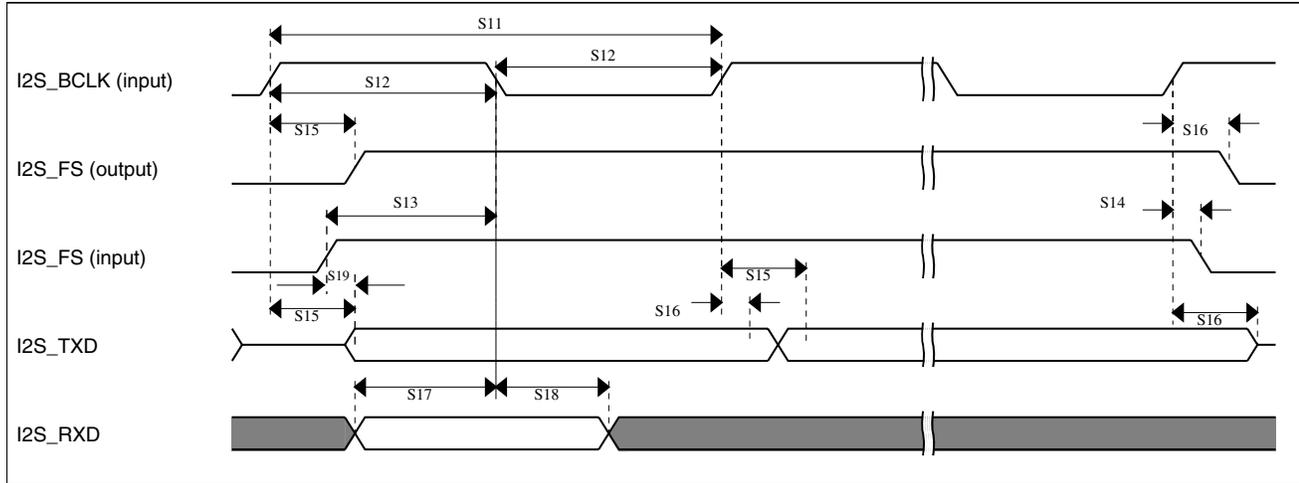
Figure 33. I<sup>2</sup>S timing — slave modes
