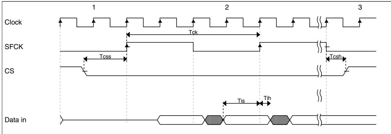
Figure 12. QuadSPI input timing (DDR mode) diagram
