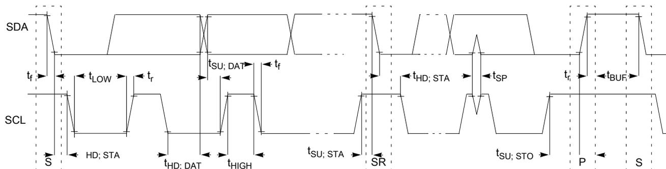
**Figure 30. Timing definition for devices on the I<sup>2</sup>C bus**
