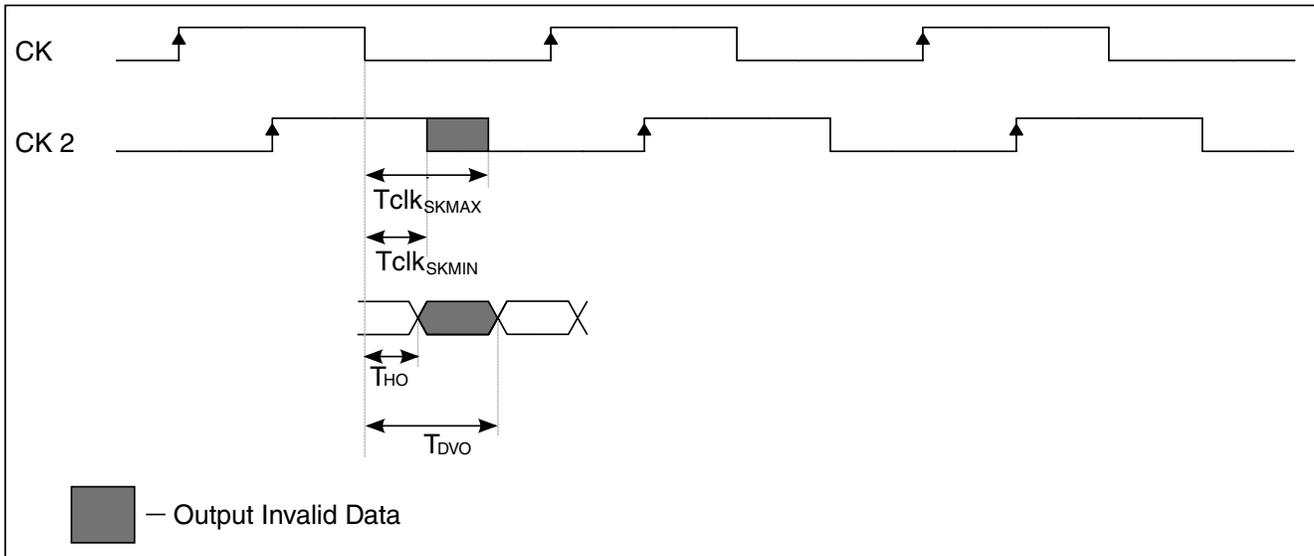
Figure 15. QuadSPI output timing (Hyperflash mode) diagram
