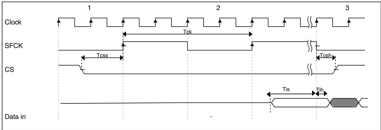
**Figure 10. QuadSPI input timing (SDR mode) diagram**
