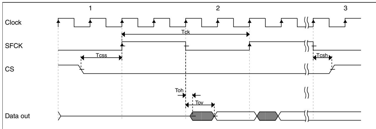
**Figure 11. QuadSPI output timing (SDR mode) diagram****Table 25. QuadSPI output timing (SDR mode) specifications**
