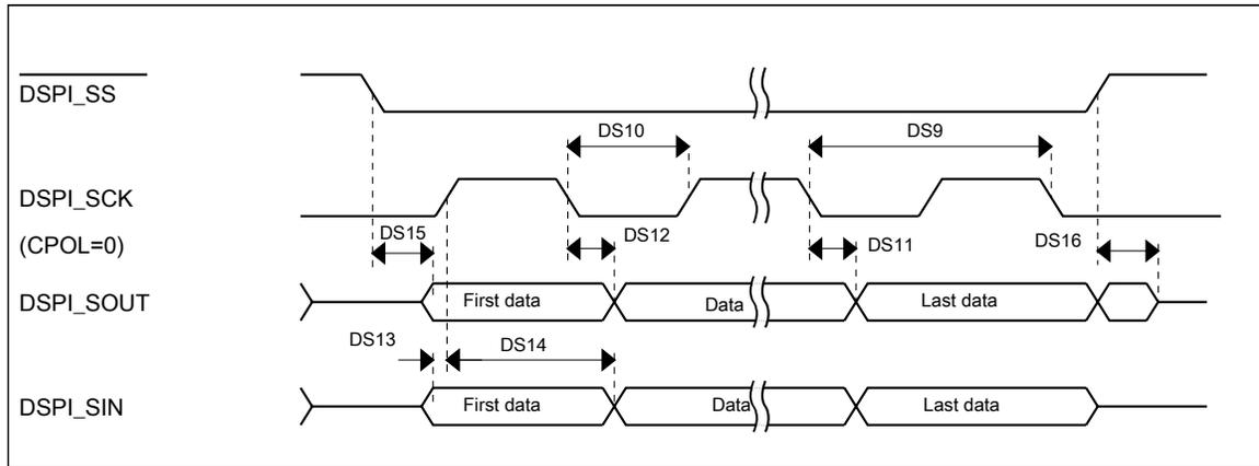
Figure 27. DSPI classic SPI timing — slave mode
