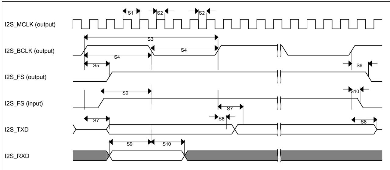
Figure 32. I<sup>2</sup>S timing — master mode
