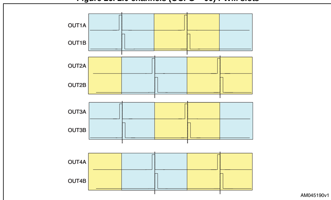
Figure 26. 2.0 channels (OCFG = 00) PWM slots
