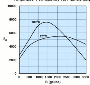
Measured on an 18/10/6mm toroid at 10kHz.
