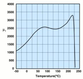
Measured on an 18/10/6mm toroid at 100kHz.
