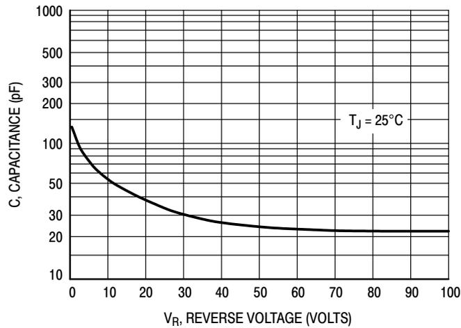
Figure 6. Typical Capacitance
