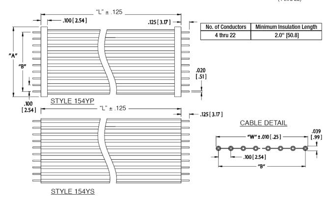
**ALL DIMENSIONS: INCHES [MILLIMETERS]** ALL TOLERANCES: ±0.005 [0.13] UNLESS OTHERWISE SPECIFIED NOT TO BE USED FOR HIGH-FLEX APPLICATIONS FOR HIGH-FLEX APPLICATIONS, SEE DATA SHEETS 11005 & 11014 CONSULT FACTORY FOR OTHER SIZES AND CONFIGURATIONS
