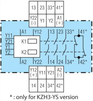
A1 (+):+/LA2:-/NY1, Y2: Feedback circuit input Y11, Y12, Y21, Y22: Control inputs (push buttons) 13, 14, 23, 24, (33, 34) \*: Safety circui outputs (forcibly guided NO contacts) (41, 42) \*: Monitoring output (forcibly guided NC contact) \*: only for KZH3-YS version
