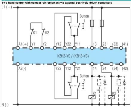
When switching inductive loads, spark absorbers are recommended
