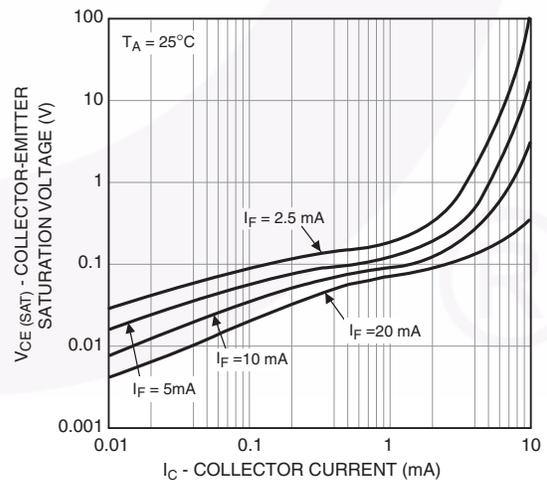
Fig. 8 Collector-Emitter Saturation Voltage vs. Collector Current
