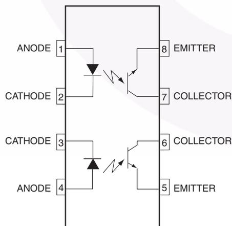
Figure 1. Schematic
