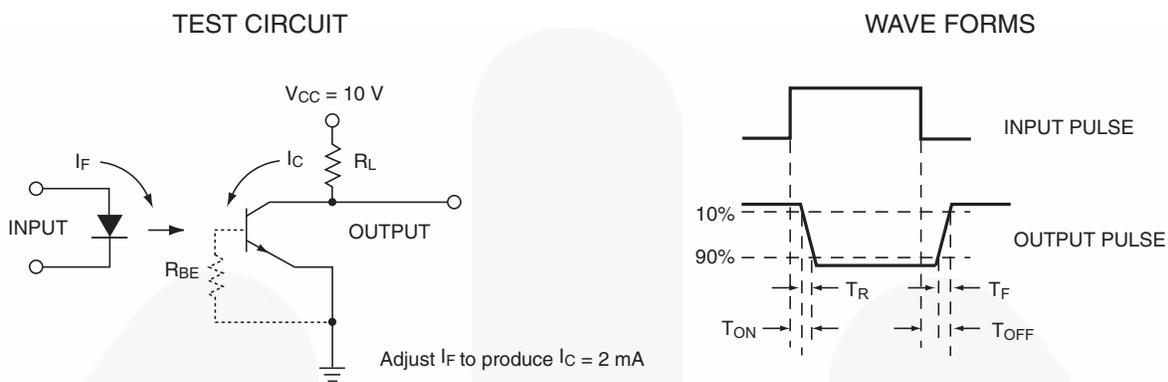
Figure 9. Switching Time Test Circuit and Waveforms
