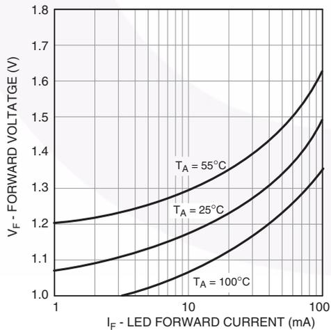
Fig. 7 LED Forward Voltage vs. Forward Current
