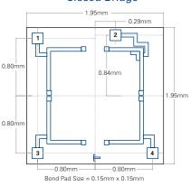
**Note:** Bridge output bond pads ( $V_{\text{-out}}$  and  $V_{\text{+out}}$ ) correspond to top side pressure. For back side pressure, the bridge outputs are reversed.
