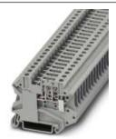
Disconnect terminal block, Connection type: Screw connection, Cross section: 0.14 mm² - 6 mm², AWG: 26 - 10, Nominal current: 20 A, Nominal voltage: 500 V, Length: 57.8 mm, Width: 6.2 mm, Color: gray, Assembly: NS 35/7,5, NS 35/15
