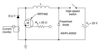
Fig. 8 - Unclamped Inductive Test Circuit
