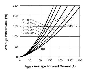
Fig. 6 - Forward Power Loss Characteristics
