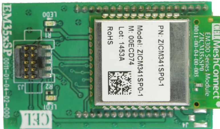
Figure 16. Module with PCB Antenna
