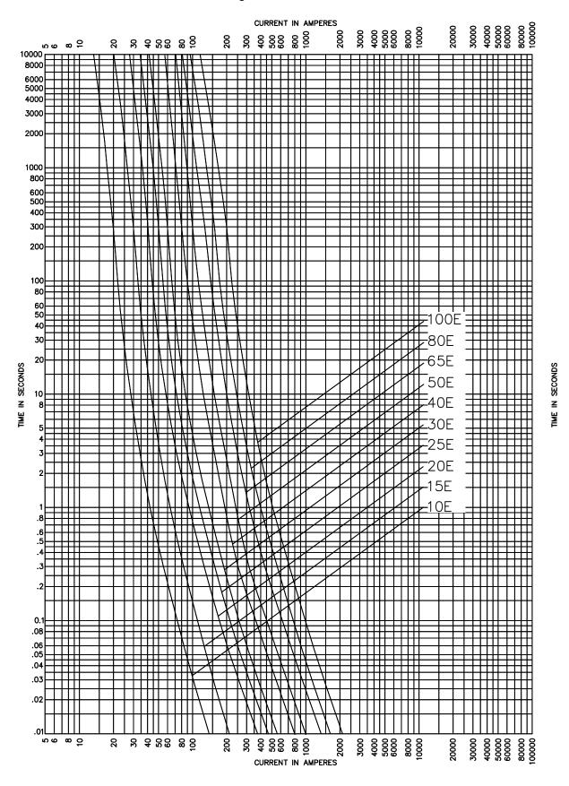
25.8 to 38 kV time-current curves — total clearing
