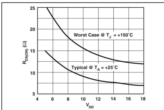
**FIGURE 2-9:** Output Resistance ( $R_{OH}$ ) vs. Supply Voltage.
