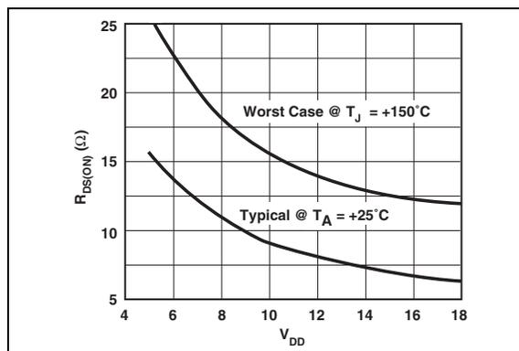
**FIGURE 2-12:** Output Resistance ( $R_{OL}$ ) vs. Supply Voltage.
