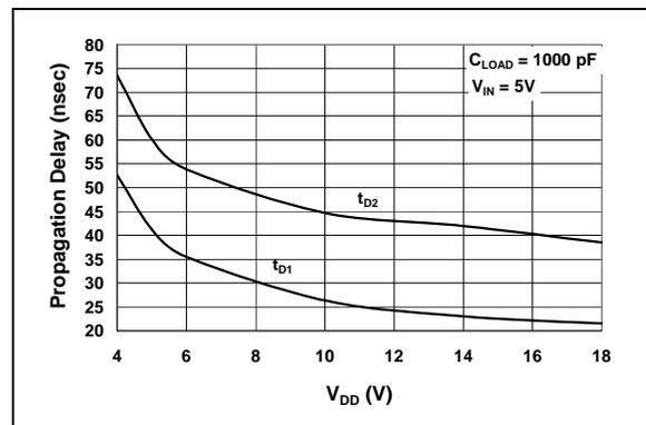
**FIGURE 2-6:** Propagation Delay Time vs. Supply Voltage.
