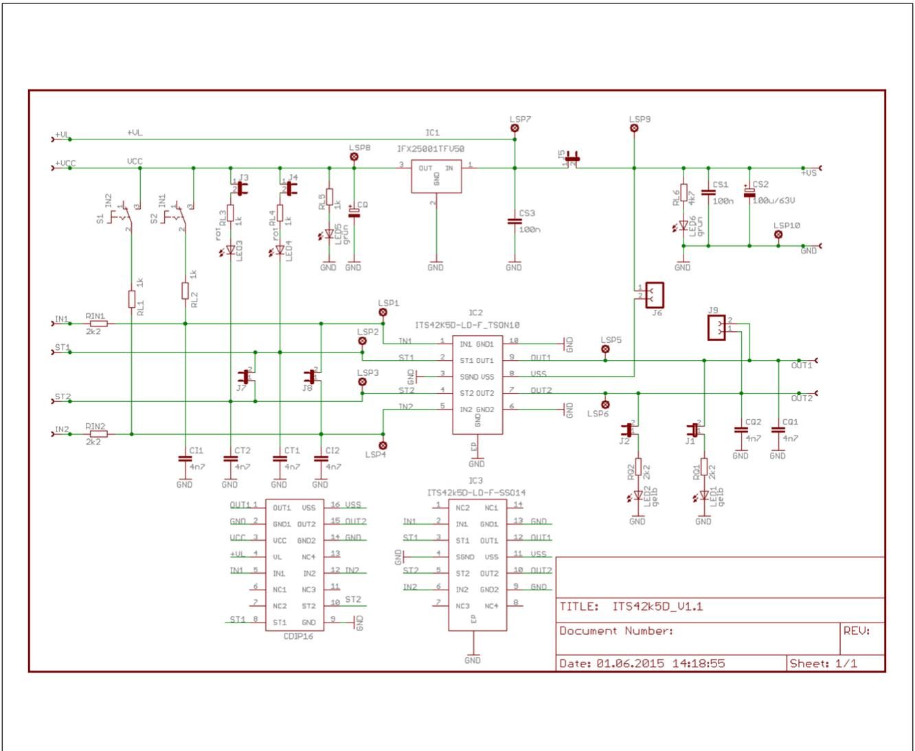
Figure 4 Schematic of ITS42k5D-LD-F Demo board (PG-TSO-10)
