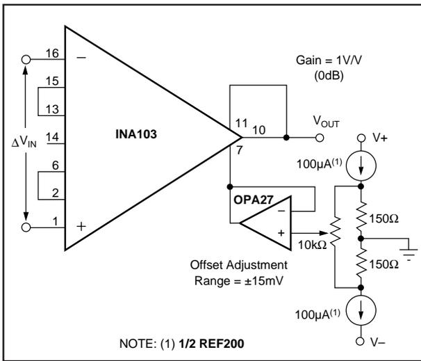
FIGURE 4. Output Offsetting.
