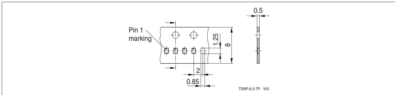
Figure 9 Tape & Reel Dimensions (reel diameter 180 mm, pieces/reel 15000)
