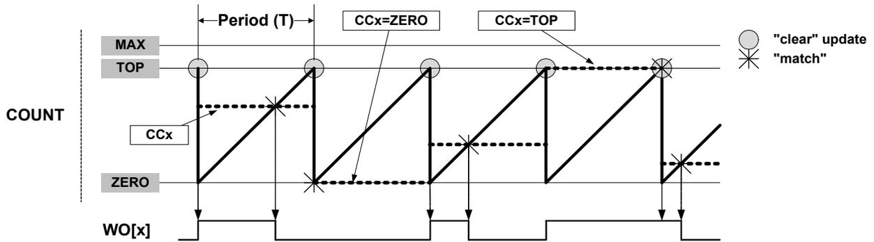
The following equation calculates the exact resolution for a single-slope PWM ( $R_{PWM\_SS}$ ) waveform:
