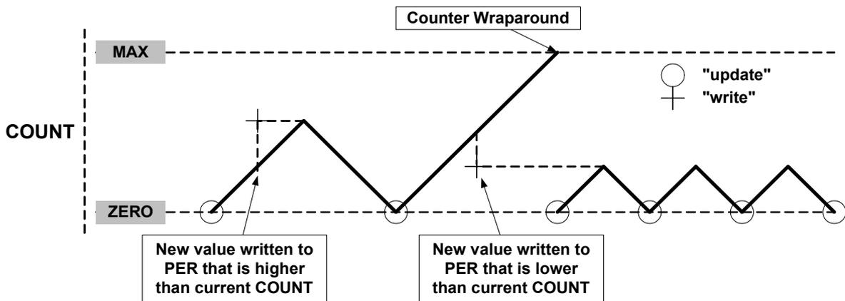
When double buffering is used, the buffer can be written at any time and the counter will still maintain correct operation. The period register is always updated on the update condition, as shown for dual-slope operation in [Figure 29-14](#). This prevents wraparound and the generation of odd waveforms.
