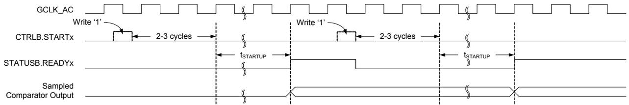
For low-power operation, event-triggered measurements can be performed during sleep modes. When the event occurs, the Power Manager will start GCLK\_AC\_DIG. The comparator is enabled, and after the startup time has passed, a comparison is done and appropriate peripheral events and interrupts are also generated. The comparator and GCLK\_AC\_DIG are then disabled again automatically, unless configured to wake up the system from sleep.
