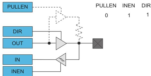
**Figure 22-8. I/O Configuration - Output with Pull**
