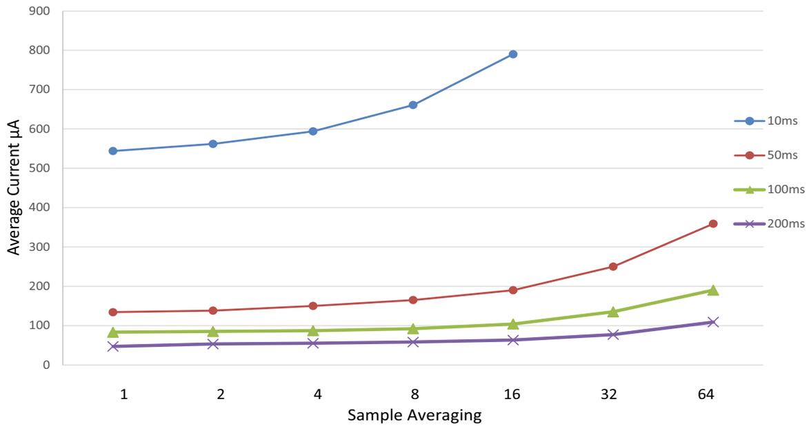
**Figure 39-10. Power consumption [ $\mu$ A].**
