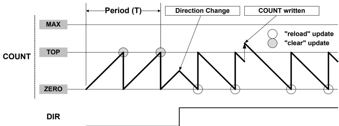
As shown in [Figure 29-4](#), it is possible to change the counter value (by writing directly in the Count register) even when the counter is running. The write access has higher priority than count, clear, or reload. The direction of the counter can also be changed during normal operation. Due to asynchronous clock domains, the internal counter settings are written when the synchronization is complete.
