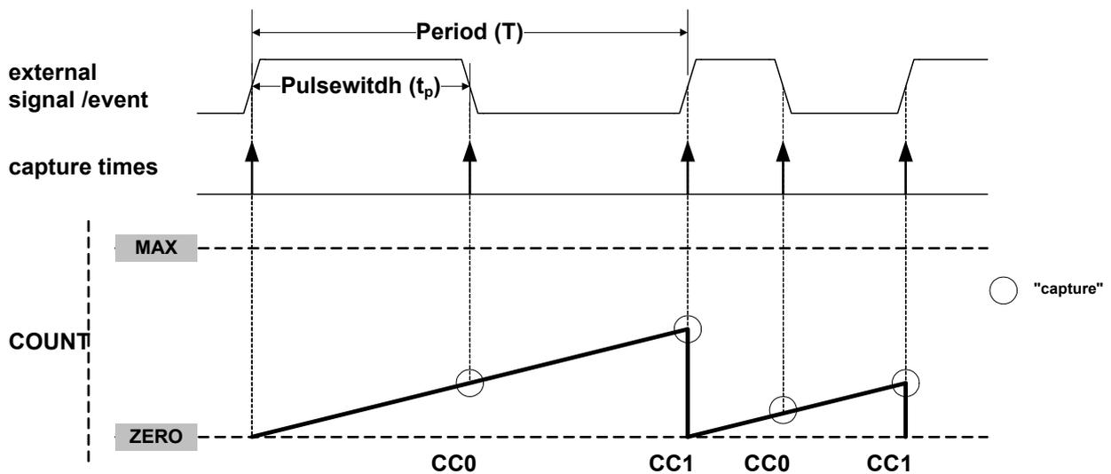
Selecting PWP or PPW in the Event Action bit group in the Event Control register (EVCTRL.EVACT1) enables the TCC to perform two capture actions, one on the rising edge and one on the falling edge.
