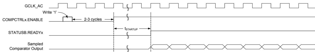
For low-power operation, comparisons can be performed during sleep modes without a clock. The comparator is enabled continuously, and changes in the state of the comparator are detected asynchronously. When a toggle occurs, the Power Manager will start GCLK\_AC\_DIG to register the appropriate peripheral events and interrupts. The GCLK\_AC\_DIG clock is then disabled again automatically, unless configured to wake up the system from sleep.
