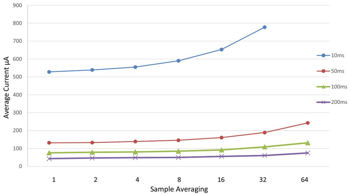
**Figure 39-9. Power consumption [ $\mu$ A].**
