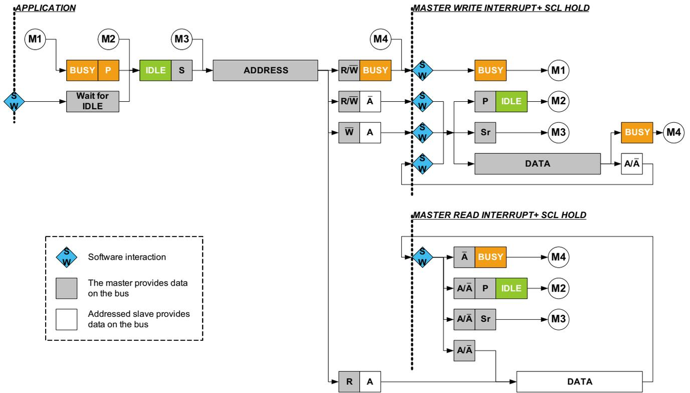
In the second strategy (SCLSM=1), interrupts only occur after the ACK bit as shown in Figure 27-7. This strategy can be used when it is not necessary to check DATA before acknowledging.
