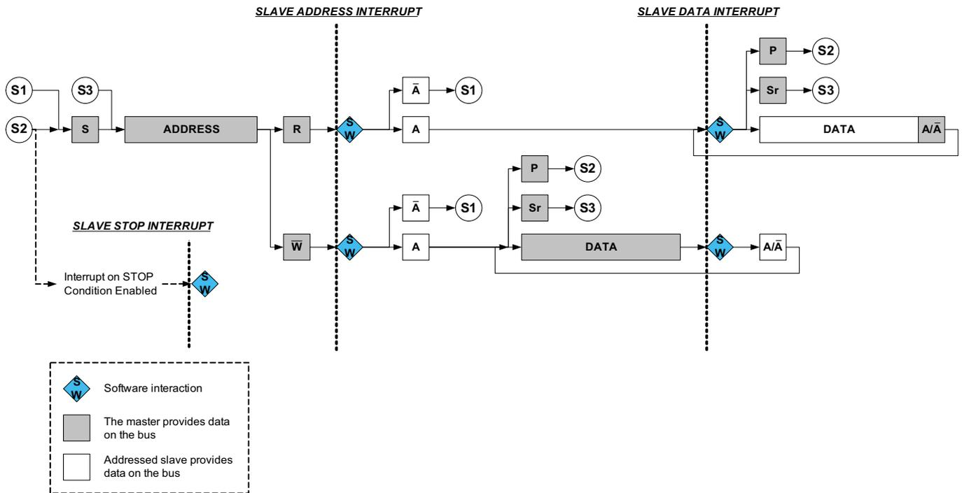
In the second strategy (SCLSM=1), interrupts only occur after the ACK bit as shown in Figure 27-11. This strategy can be used when it is not necessary to check DATA before acknowledging. For master reads, an address and data interrupt will be issued simultaneously after the address acknowledge, while for master writes, the first data interrupt will be seen after the first data byte has been received by the slave and the acknowledge bit has been sent to the master.
