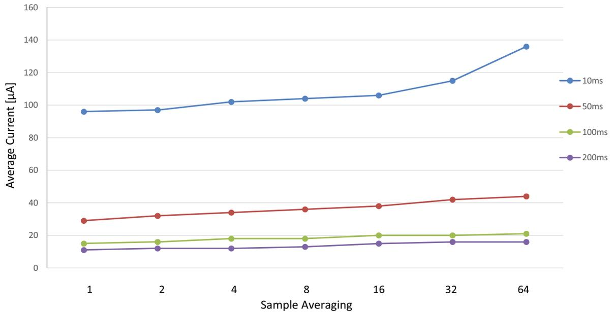
**Figure 39-7. Power consumption [ $\mu\text{A}$ ].**
