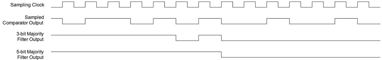
**Figure 31-7. Single-Shot Filtering**
