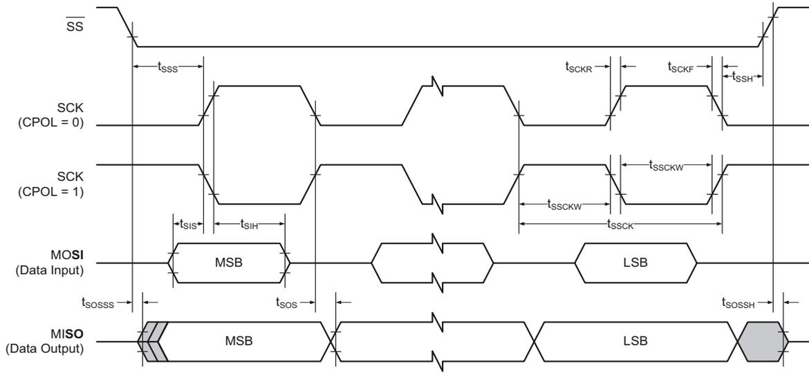
**Table 39-44. SPI timing characteristics and requirements<sup>(1)</sup>**
