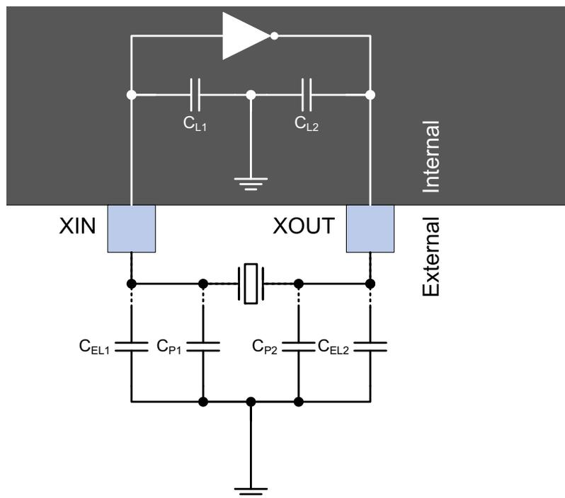
Using this model the total capacitive load for the crystal can be calculated as shown in the equation below:
