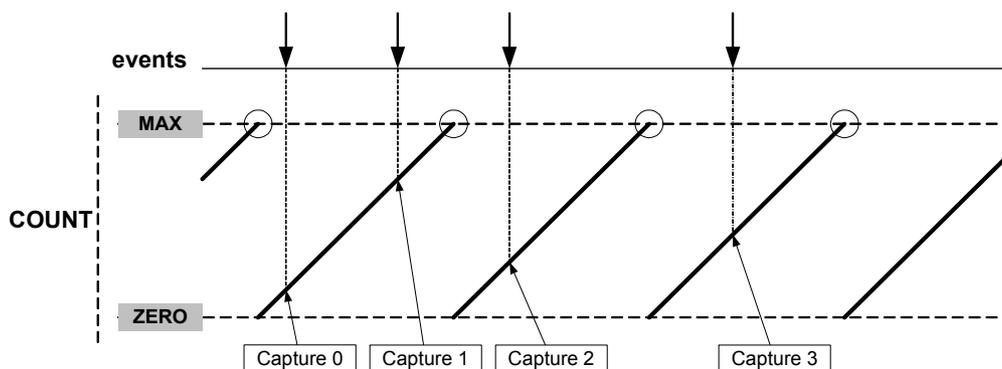
For input capture, the buffer register and the corresponding CCx act like a FIFO. When CCx is empty or read, any content in CCBx is transferred to CCx. The buffer valid flag is passed to set the CCx interrupt flag (IF) and generate the optional interrupt, event or DMA request.
