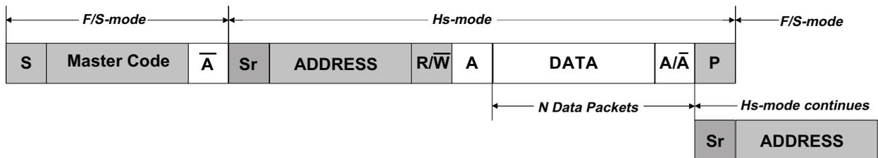
Transmitting in High-speed mode requires the I2C master to be configured in High-speed mode (SPEED=0b10) and the SCL clock stretch mode (SCLSM) bit set to one.
