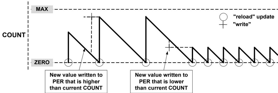
A counter wraparound can occur in any mode of operation when up-counting without buffering, as shown in [Figure 29-11](#). This is due to the fact that COUNT and TOP are continuously compared, and if a new value that is lower than the current COUNT is written to TOP, COUNT will wrap before a compare match happens.
