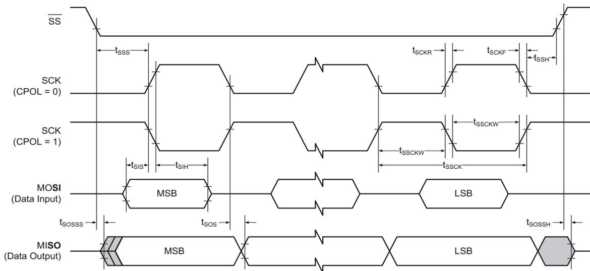
**Table 34-47. SPI timing characteristics and requirements<sup>(1)</sup>**
