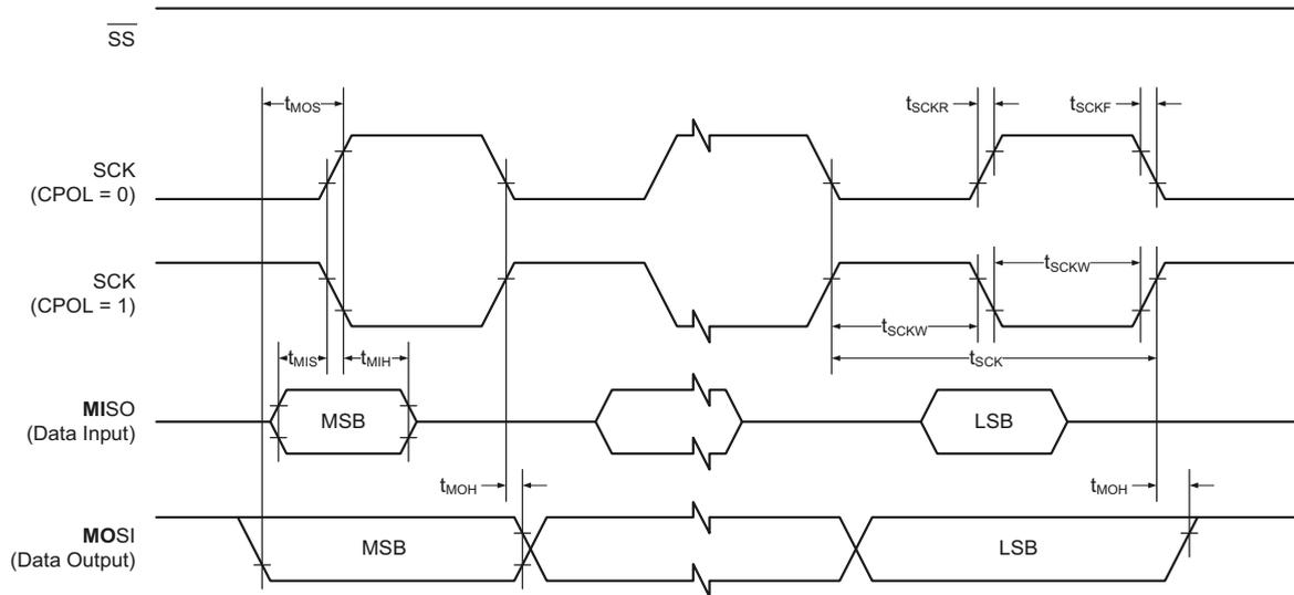
Figure 34-15. SPI timing requirements in slave mode
