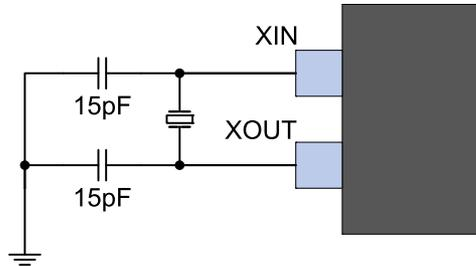
The crystal should be located as close to the device as possible. Long signal lines may cause too high load to operate the crystal, and cause crosstalk to other parts of the system.
