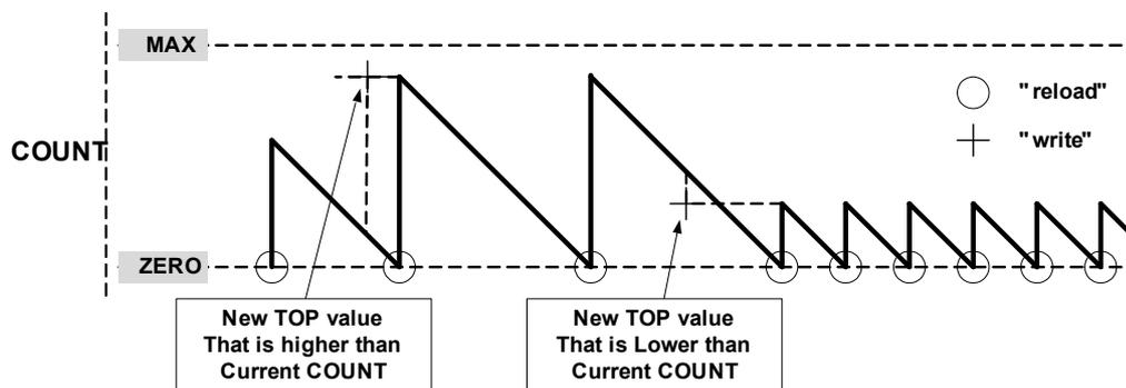
When counting up a change from a top value that is lower relative to the old top value can make the counter miss this change if the counter value is larger than the new top value when the change occurred. This will make the counter count to the max value. An example of this can be seen in [Figure 28-8](#).
