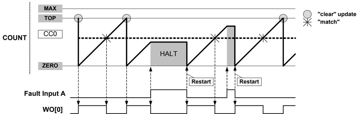
Figure 29-30. Waveform Generation with Fault Qualification, Halt and Restart Actions
