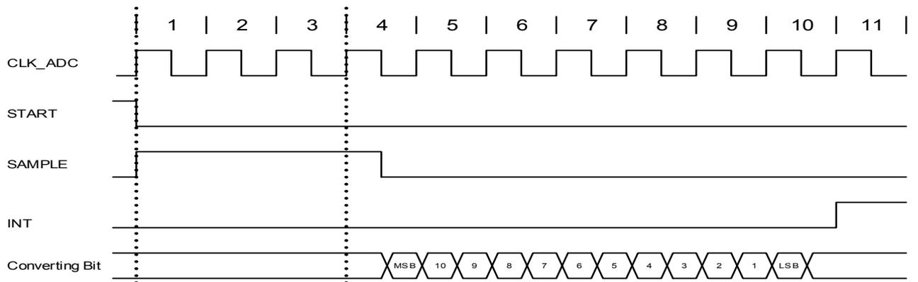
**Figure 30-5. ADC Timing for Free Running in Differential Mode without Gain**
