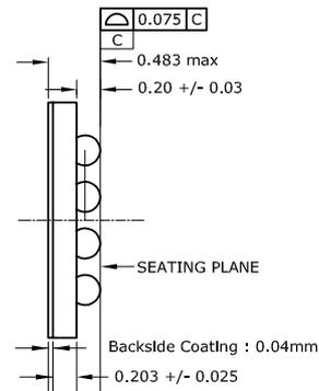
Notes : 1. Dimension "b" is measured at the maximum ball diameter in a plane to the seating plane.
