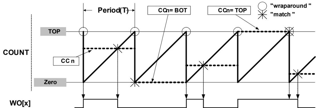
In match operation, Compare/Capture register CC0 is used as the top value, in this case a negative pulse will appear on WO[0] on every overflow/underflow.
