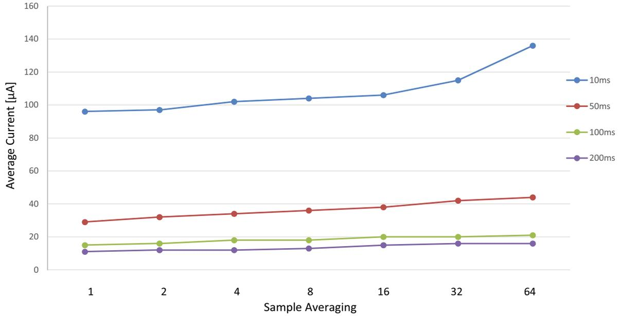
**Figure 34-8. Power consumption [ $\mu\text{A}$ ].**
