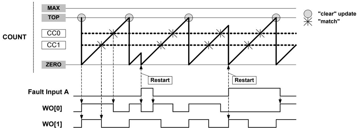
Figure 29-26. Waveform Generation in RAMP2 mode with Restart Action
