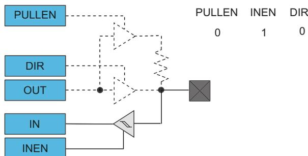
**Figure 22-5. I/O Configuration - Input with Pull**
