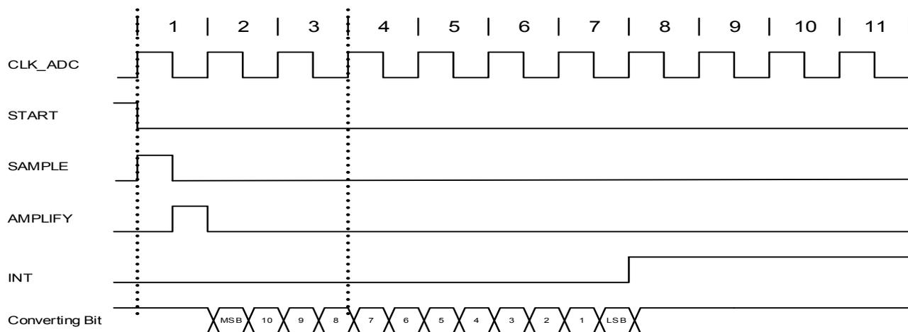
**Figure 30-7. ADC Timing for Free Running in Single-Ended Mode without Gain**
