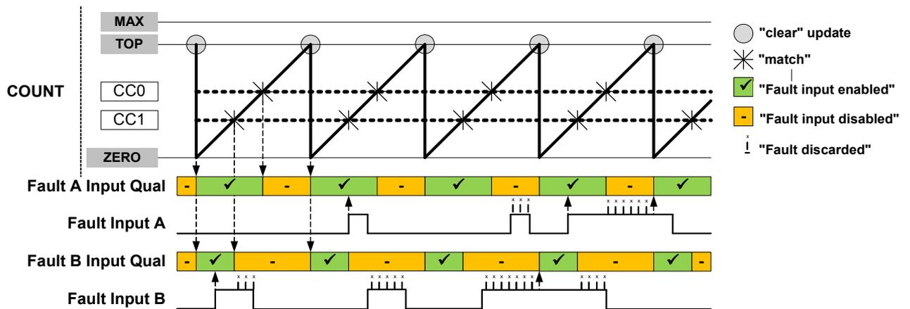
Figure 29-23. Fault Qualification in RAMP2 Operation with Inverted Polarity
