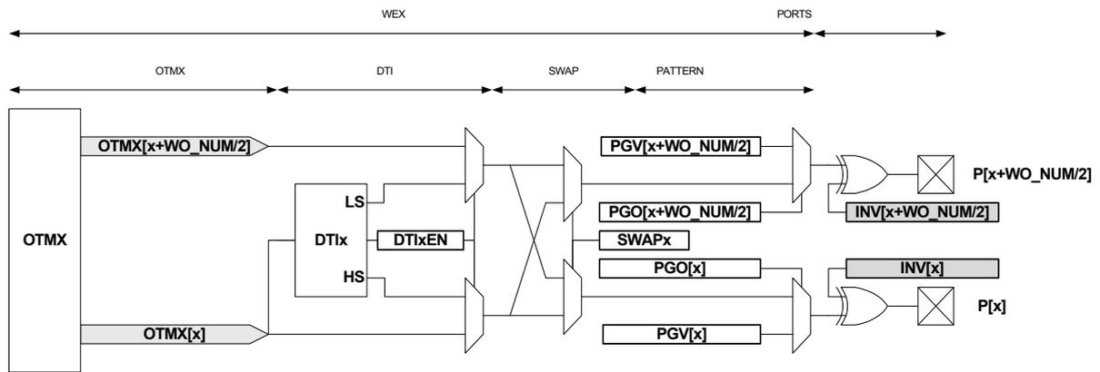
The output matrix (OTMX) unit distributes compare channels, according to the selectable configurations, as shown in Table 29-4.
