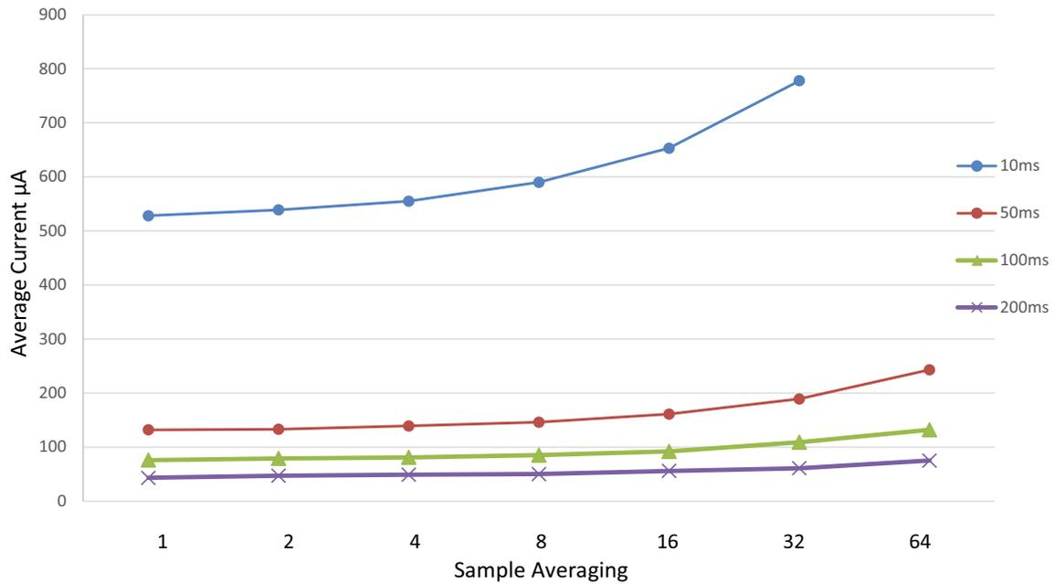
**Figure 34-10. Power consumption [ $\mu\text{A}$ ].**
