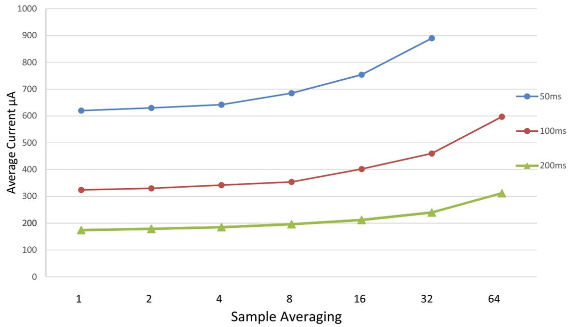
**Figure 34-12. Power consumption [ $\mu\text{A}$ ].**
