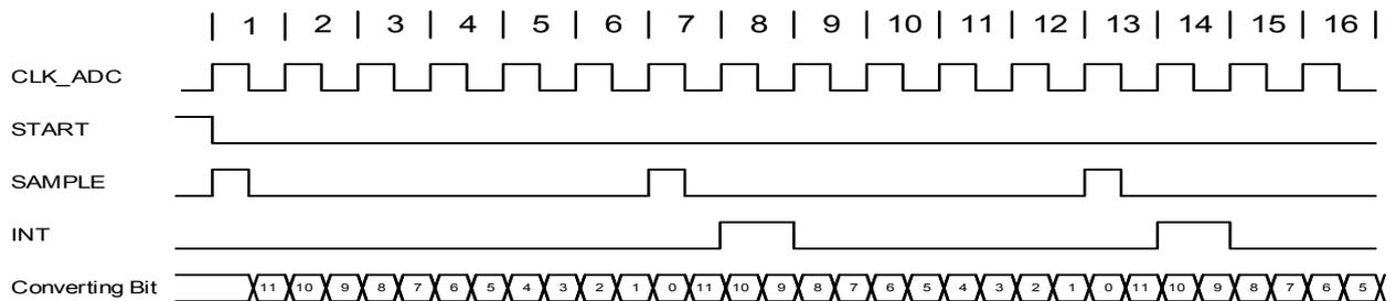
**Figure 30-6. ADC Timing for One Conversion in Single-Ended Mode without Gain**
