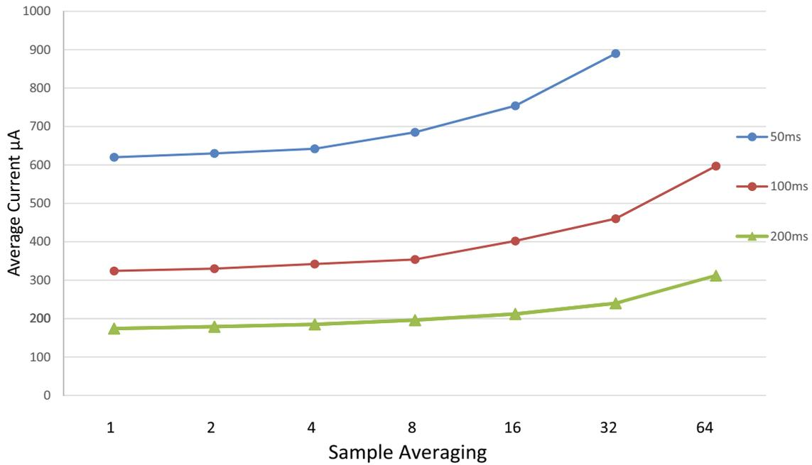
**Figure 39-11. Power consumption [ $\mu$ A].**
