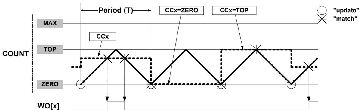
Using dual-slope PWM results in a lower maximum operation frequency compared to single-slope PWM generation.
