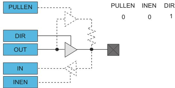
**Figure 22-7. I/O Configuration - Totem-Pole Output with Enabled Input**
