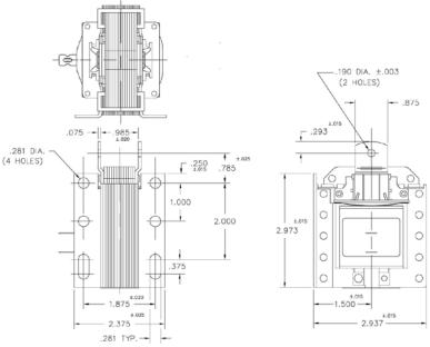
Solenoid shown energized in drawing with plunger fully seated
