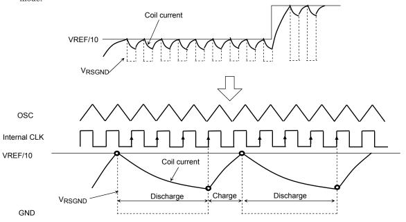
(3) Operation on change of predetermined current value (when in Discharge mode) The TB6569FG enters Discharge mode as  $V_{RSGND}$  reaches the predetermined voltage (VREF/10) and then transits to Charge mode after four internal clocks. However, if  $V_{RSGND} > V_{REF/10}$  at the time, the TB6569FG goes back to Discharge mode. If  $V_{RSGND} > V_{REF/10}$  after another four internal clocks, then the TB6569FG enters Charge mode and stays until  $V_{RSGND}$  reaches  $V_{REF/10}$ .
