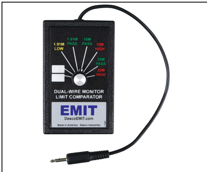
Figure 5. EMIT 50524 Limit Comparator for Dual-Wire Monitors
