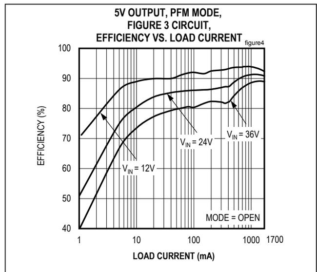
Figure 4. MAX17545 5V Output Efficiency (PFM Mode)
