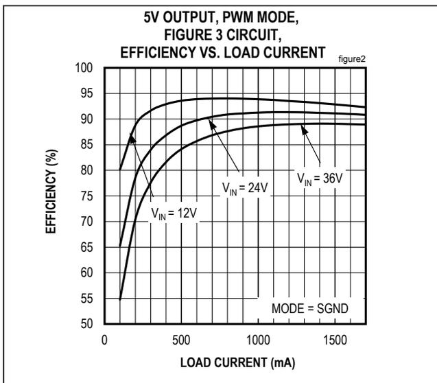
Figure 2. MAX17545 5V Output Efficiency (PWM Mode)
