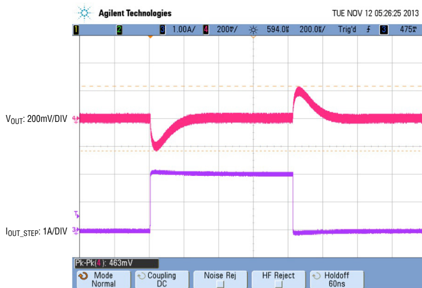
Figure 7. Measured Channel 3 Load Transient V_{IN} = 24V , V_{OUT3} = 12V , I_{STEP} = 0A to 2A I_{STEP} Slew Rate = 1A/\mu s
