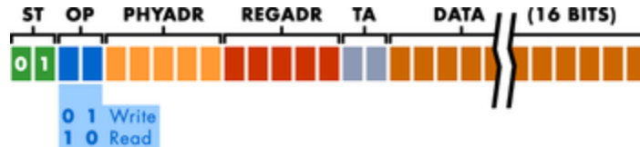
Figure 27 : Basic MDIO Frame Format
