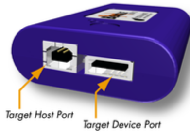
Figure 36 : Beagle USB 12 Protocol Analyzer - Capture Side
