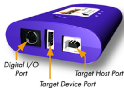
Figure 32 : Beagle USB 480 Protocol Analyzer - Capture Side
